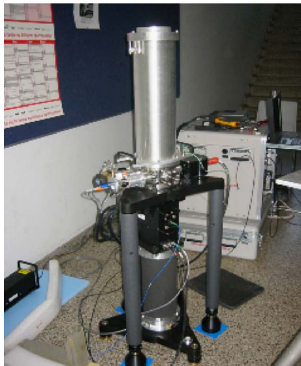
Fig. 1. Absolute gravimeter (FG-5), capable of 10^{-9} accuracy during a 1–2-day measurement. Local environmental effects are the main limitation in accuracy of such measurements.
